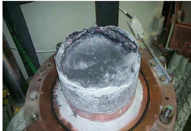
Figure 6. Solidified electrolyte and cathode.
