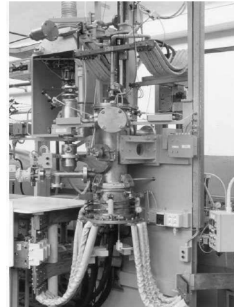
Figure 2. GTT High temperature electrowinning cell.
