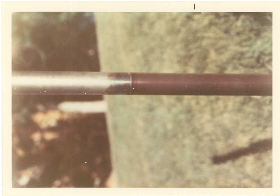
Fig. 10A - After 180 minutes at 14.5 volt and 0.12 amp.
