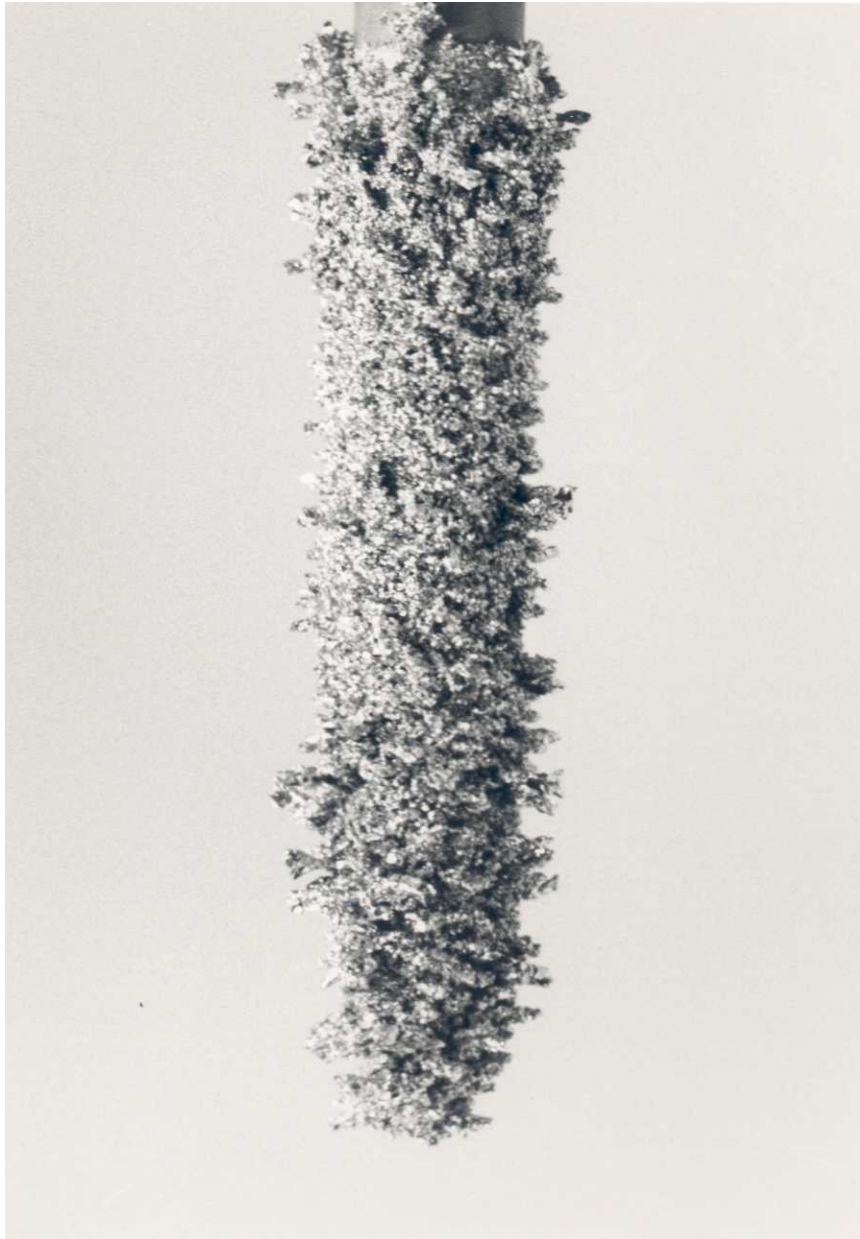
Fig. 21 - Deposit obtained under ultrasonic vibration and low temperature.
