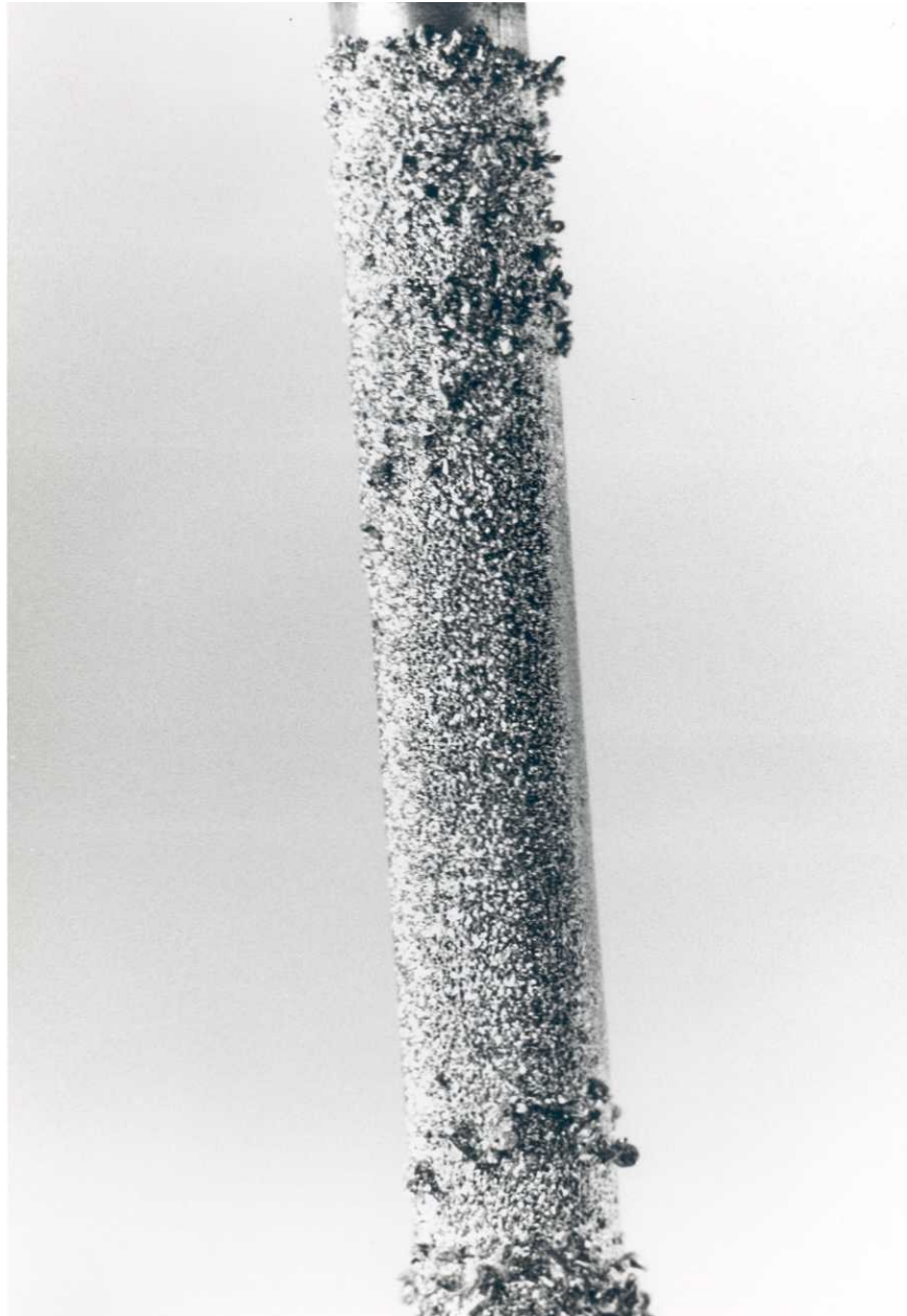
Fig. 10 - Deposit resulted with pulsating current.
