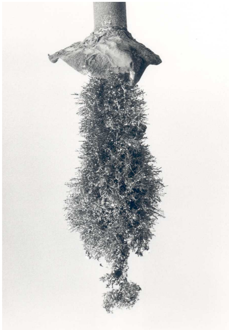
Fig. 13 - Whiskers obtained with a periodically reversed current without dead time.
