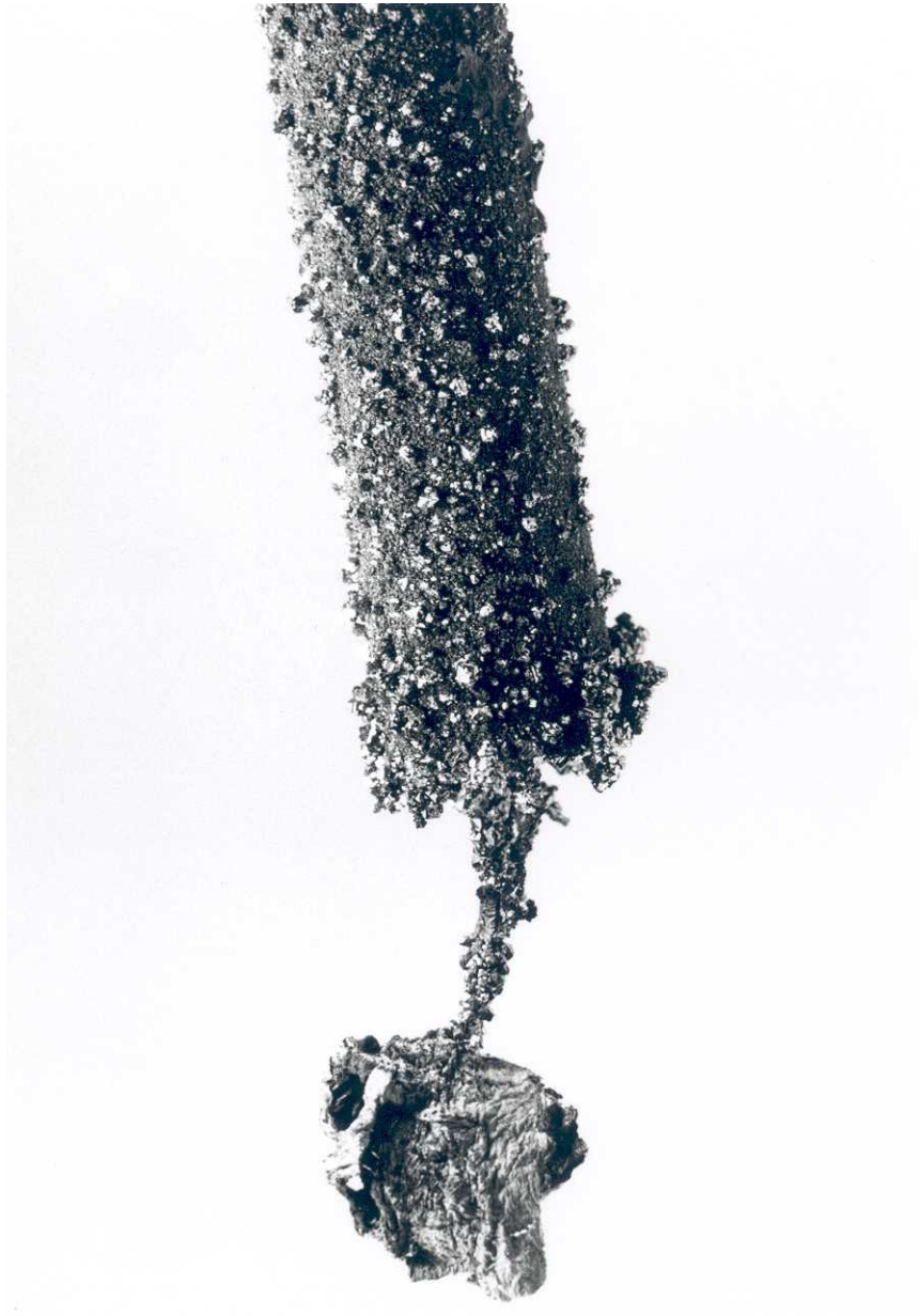
Fig. 20 - CER deposit obtained simultaneously with the ultrasonic vibrated cathode shown in Fig. 18.
